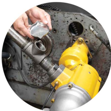
Brutal lab testing featuring steel shot in the starter's inlet line demonstrates rugged reliability
