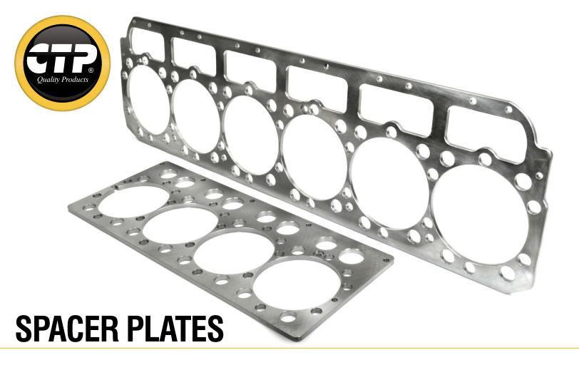
Engine block spacer plates were designed to reduce stresses on the liner flange, which could cause it to get cracked. The spacer plate is just a few thousands of an inch thinner than the liner flanges, this ensures the correct liner protrusion and guarantees proper head gasket sealing.
