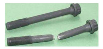
Used TTY (Torque-To-Yield) head bolts will snap in the process of re-torqueing the cylinder head. If they do not snap, the already permanently stretched bolts will stretch even further and rapidly lose clamping load. The loss of clamping load could ultimately lead to head gasket failure.
