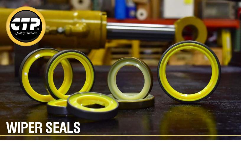
The main function of the **Wiper Seals**, also known as **Dust Seal**, is to keep the rod and cylinder clean and free from dirt and debris as it retracts; thus preventing early breakdown.
